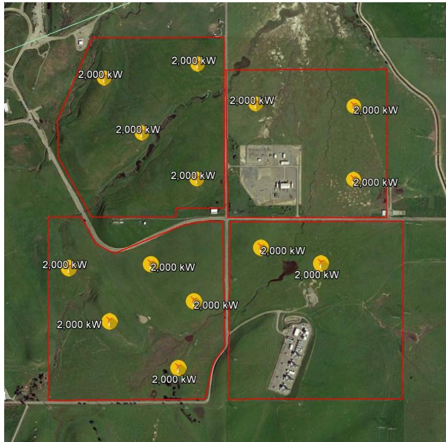
*Figure 4 - Mountain House turbine placement detail*
